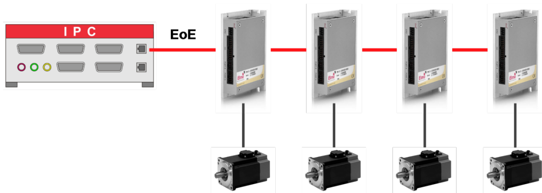
Figure 15: TwinCAT and EAS EoE Configuration
